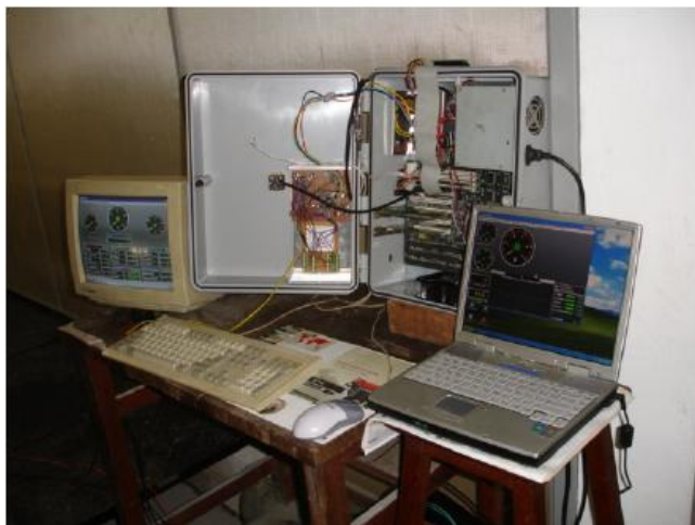
Figure 23. Data acquisition system Source: CENBIO, 2008
